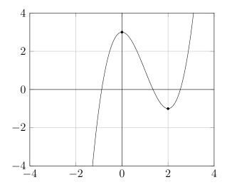
Just by looking at the graph, we can see the two points where the derivative of f is zero (i.e., the two points where the tangent lines are horizontal). They roughly occur at x = 0 and x = 2. (And you can prove that they *exactly* occur there if you do out the math—that is, if you solve the equation f'(x) = 0 for x.)
