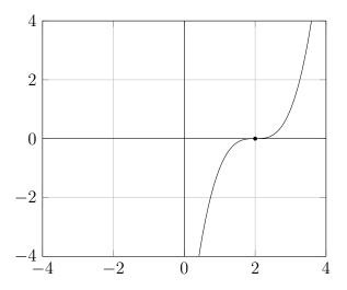
This is a strange example, but it is a great one. As you can see, the graph does have "flat" tangent line at x = 2, but x = 2 is neither a local maximum nor a local minimum—I can immediately get larger than f(2) = 0 by moving right, or immediately get smaller than f(2) = 0 by moving left.
